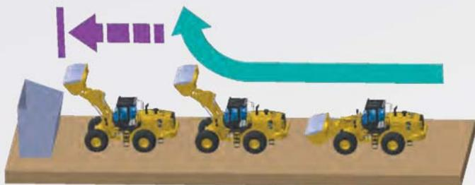
Shift change delay mode is provided to avoid an excessive rise in travel speed during digging and loading. When moving forward with the lift arm up, the second gear is kept for eight seconds to prevent over-speed. When reversing, the second gear is kept for eight seconds. These delays to third gear help to keep fuel consumption down ensuring smooth loading.
